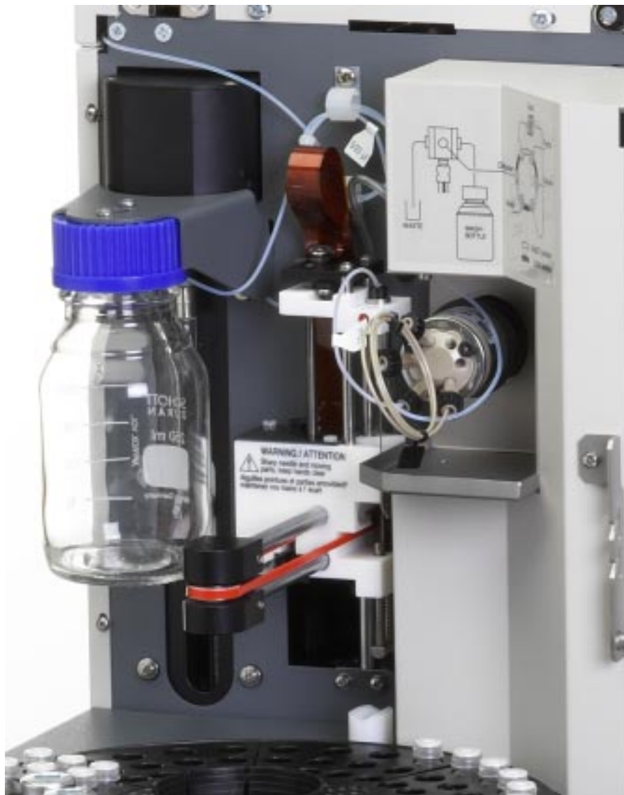
Close-up showing the switching valve, the lift mechanism as well as the bottle for the rinsing solution
