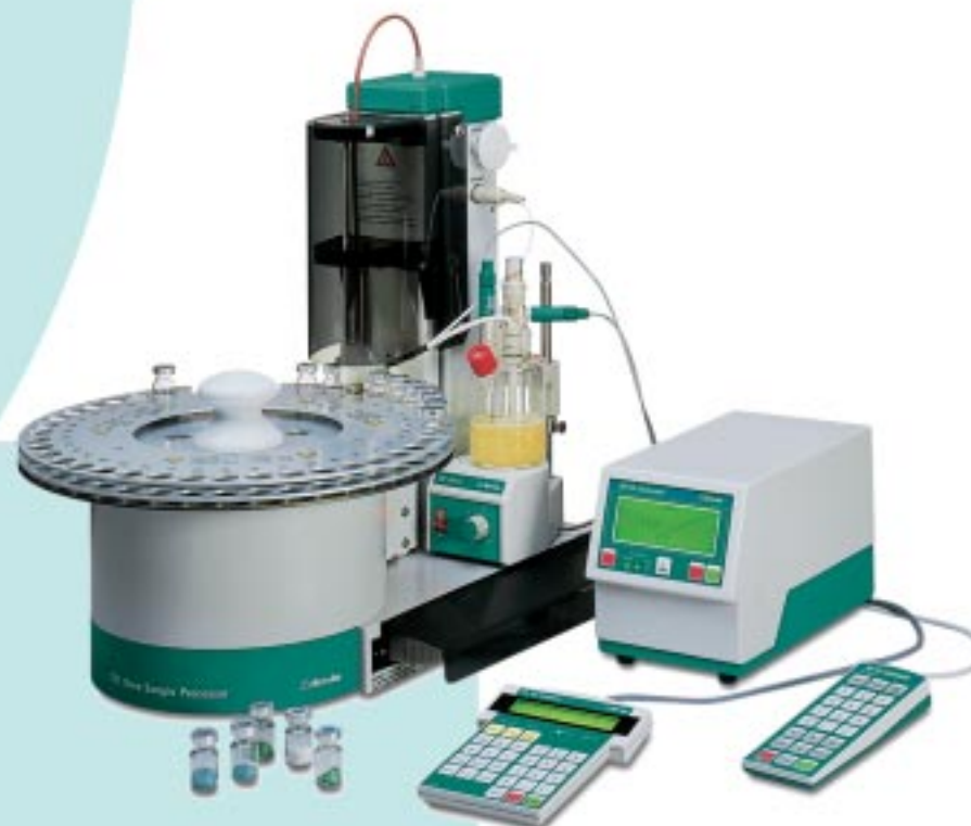
831 KF Coulometer with 774 Oven Sample Processor: fully automated, fast and highly precise KF water determinations right down to the trace level.
