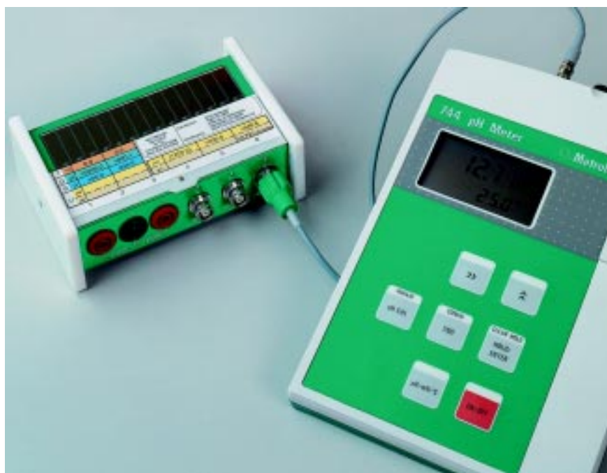
Checking the pH display of a 744 pH Meter with the Calibrated Reference.
